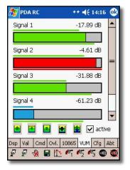
A level meter display with min. and max indicators is also on the PDA available. To take care about the PC's system resources it is possible to de-activate this feature. To signal unsuited input ranges immediately, the colour of the level display changes depending on the level's range. For every channel the display shows the signal name and the level relative to the maximum input rang level.
