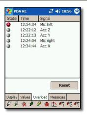
The Pocket PC logs the overload information from PULSE's input channels, displaying the results in a separate list. Not only the channel, but the time at which the overload occurred is shown. Recently overloaded channels are denoted by greyed icons until the channel is reset.
