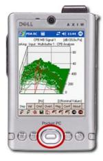
The cursor of a display can be shifted with the help of the direction keys of the navigation jack in x and z-direction. That has also influence on the values of the cursor value dialog field, if the "Cursor Value" is indicated for this display. On the other hand, a cursor value
