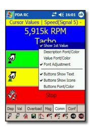
Along with the option of controlling the measurement via the standard GUI controls of the PULSE system, PDARemotePULSE allows the setup of a dedicated GUI with just a few large buttons for the major controls. This makes it possible to operate PDARemotePULSE as a touch pad using ones fingers.
