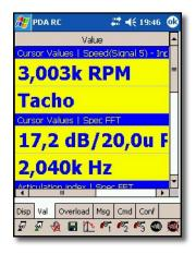
Together with the displays that are available from PULSE, it is possible to display a range of cursor values, thanks to the PDARemotePULSE integrated server component inside of the PULSE software. These values are shown within their own display on the Pocket PC and continually updated in the same way as the displays.
